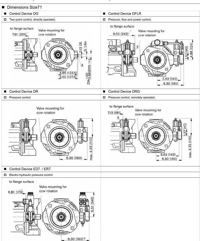
1) ER7.: 7.68 inches (195 mm) if using a sandwich plate pressure reducing valve.
