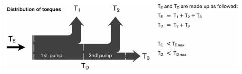
□ A through drive with U shaft is also possible if these conditions are observed and technical data is reduced, whereby T<sub>E max</sub> apuals T<sub>D max</sub>, please contact us.
