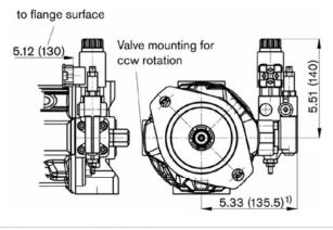
1) ER7.: 6.71 inches (170.5 mm) when using a sandwich plate pressure reducing valve. For details of connection options and drive shafts, see also above data.
