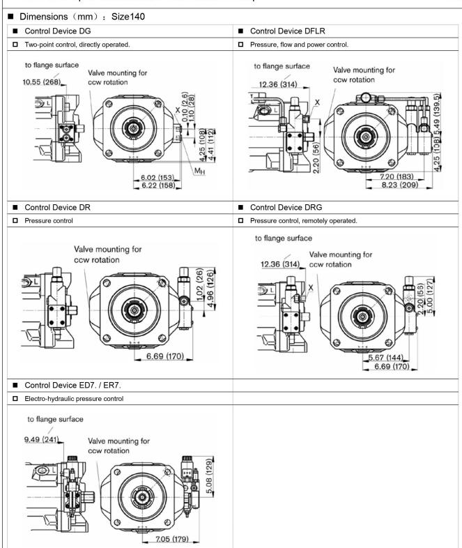
1) ER7.: 214 mm when using a sandwich plate pressure reducing valve.
