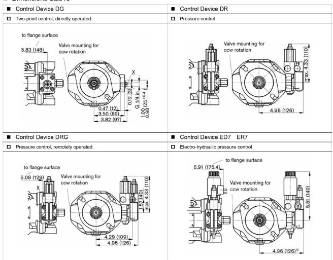
1) ER7.: 6.34 inches (161 mm) if using a sandwich plate pressure reducing valve.
